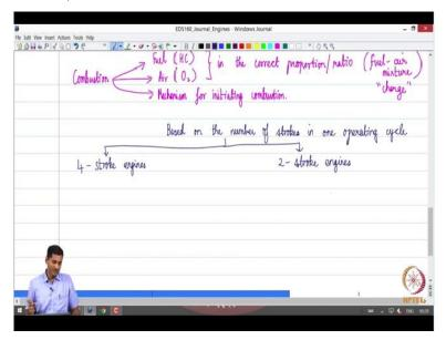
So, another criteria for classifying IC engines is based on the number of strokes in one operating cycle okay. So of course in our course we will consider both spark ignition and compression ignition engines okay, we are going to look at both right. So, we look at what is an operating cycle and what do we mean by stroke and so on right as we go along. So, based on this criteria we have what are called as 4 stroke engines and 2 stroke engines.
