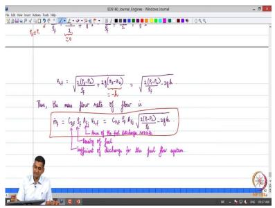
Please note that CDf is the coefficient of discharge for the fuel flow system ok. Rho f is the density of fuel ok Afj is the area of the fuel discharge nozzle ok at the tip ok that is Afj ok. So these are the various parameters.
