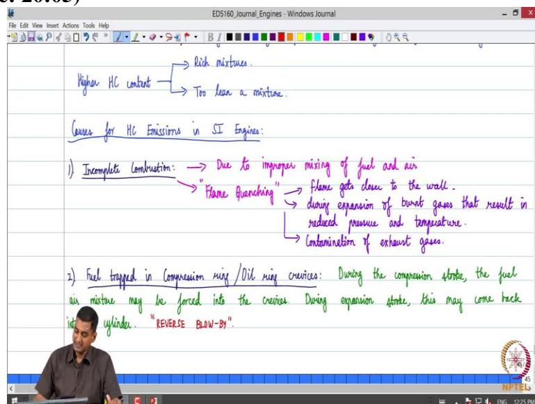
And what factors are result in significant hydrocarbon emissions. So, the first one is due to incomplete combustion obviously. So, the combustion process is not incomplete needs to not
