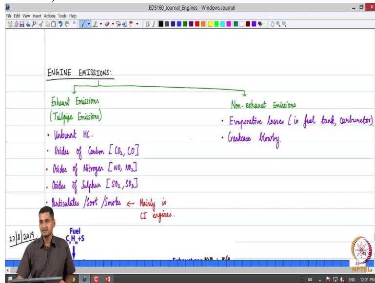
Greetings so start let us start get started with today's class. So, looking at engine emissions, so broadly emissions from IC engines you know like, can be classified as what are called exhaust emissions that come from the tailpipe, which include all these gases unburned hydrocarbons, Oxides of carbon Oxides of nitrogen, Oxides of Sulphur and also like emissions in the form of particularly particulate matters.
