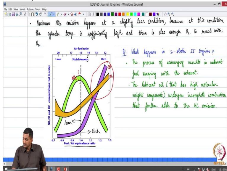
So that is when the NOx emissions become the highest of course typically, maximum NOx emission or happens at a slightly lean condition. So, if you compare it, happens at a slightly lean condition because at this condition the cylinder temperature is sufficiently high and there is enough excess oxygen also so, we need oxygen to reactive nitrogen so if you have exactly stoichiometric so there is only enough oxygen to react to the hydrocarbon and oxidize them.
