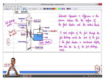
So let is get started. So a quick recap of where we stopped this. In the last class, we were looking at the simple carburetor and this is a schematic of the same. So, we have had taken from the atmosphere entering to the section labeled as a prime and that flows through venturi which is a restriction in the cross section and the pressure drop when the air flows through the venturi and the pressure drop is a maximum when the throat of the venturi and there the as speed will be the highest.
