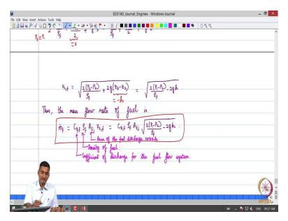
So now let us apply the Bernoulli's equation for the flow of fuel. So, if we apply the Bernoulli equation for the flow of fuel, please know that I we are going to apply the Bernoulli equation between the throat section and the top surface of the fuel in the flow chamber. So those are the 2 points between which we are going to apply the Bernoulli equation. So if we apply the Bernoulli equation what is going to happen we will get P3 by rho f + V2 f square.
