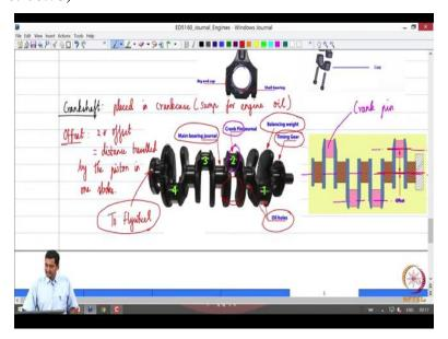
What are called as crank pins journals, this is what is called a crank pin okay. So this the crankshaft, the piston essentially, is connected to the crankshaft. And this connecting this end of the connecting rod rests on the crank pin okay, it is mounted through some bearings, okay. So you can see a very simple 2D diagram. So this is the axis of rotation of the crankshaft, let us say the central axis.
