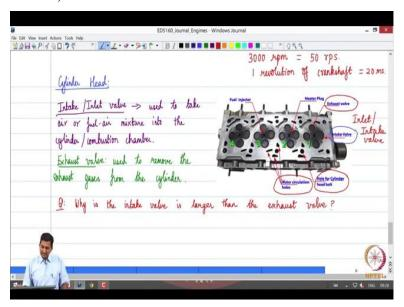
So we have looked at the cylinder block, the crankcase, now let us go to the cylinder head okay, so that is the other that is the third chunk block as far as the 4 stroke engine is concerned, right. So, what happens in the cylinder head this is a bottom view of the cylinder head. So, imagine that you flip the cylinder head, place it on top of the cylinder block and then bolted okay using a gasket in between to prevent liquids right.
