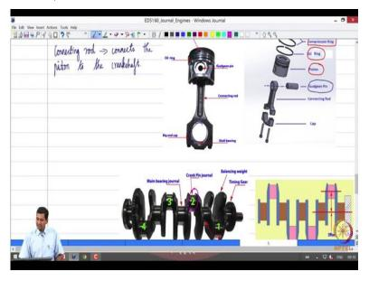
So, let us build on from there and then like let us look at more components today okay. So, the next important component in the which is fit within the cylinder block is the piston. So, the piston is a component you know, like on which the what to say the forces that are generated due to the conversion process act and the thermal energy is converted to kinetic energy okay. So that way it is a very important component in an internal combustion engine.
