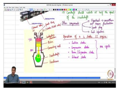
So, these are some of the main components, some other components which we would also discuss as we go along one would be what is called as a flywheel, okay. A flywheel is nothing but a mass, which is attached to the output of the crankshaft. The crankshaft is the link which comes out of the engine and it provides the tractor effort to drive the wheels and propel the vehicle.
