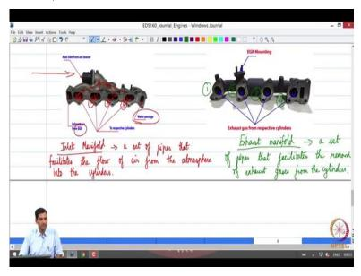
So we looked at the intake manifold and the exhaust manifold which are nothing but mechanisms that aid in this process.
