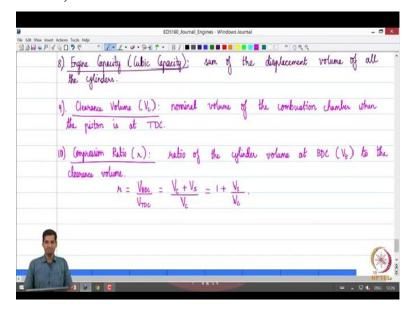
The engine capacity or cubic capacity is the sum of the displacement volume of all the cylinders okay. So that is the engine capacity or the cubic capacity. Of course, if a single cylinder engine, just what it is, right. If you have a multi cylinder engine, you need to add the sum of the displacement volumes of each cylinder. So let us say if I say I have an engine in a car with a capacity of 1.2 liters.
