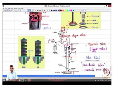
So we looked at what was called as valve float, which happens and typical spring rate and valves at high speeds and how it can be minimized and how you know one could eliminate it by using a desmodromic valve. So, that is where we stopped yesterday.
