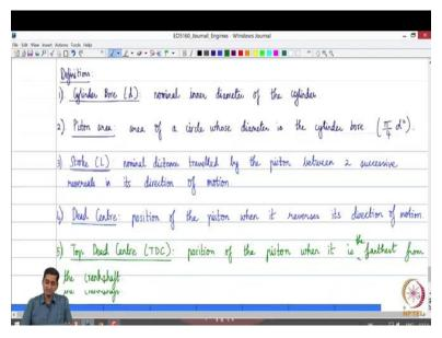
So before we go and look at these 4 strokes in detail I am just going to write down a few definitions concerned with what to say engines in this okay. So the first one is what is called as a cylinder bore okay let me indicate it by a parameter d okay. This is the nominal inner diameter of the cylinder or the combustion chamber okay. So, the cylinder bore is nothing but the nominal inner diameter of the combustion chamber or a cylinder okay.
