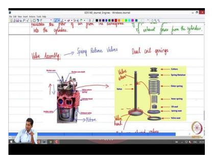
And we also looked at the valve assembly, which in most automobiles you know it is a spring return valve wherein a dual coil spring is used to close the valve once the what to say corresponding processes completed either the intake or the exhaust process, okay.
